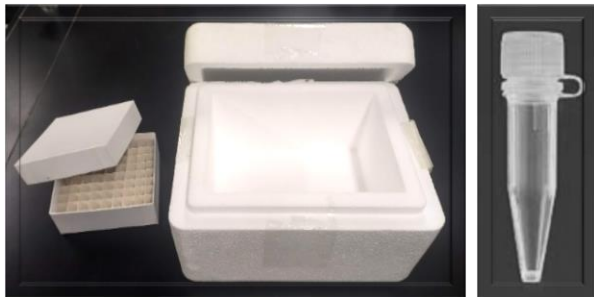
From left to right: cardboard freezer box with 81-cell divider; foam shipping cooler; 1.5 mL round bottom tether cap tube.
